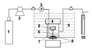
Fig. 5 Schematic diagram of the experimental apparatus: (1)  $CO_2$  cylinder; (2) syringe pump; (3) pressure gauge; (4) stainless steel autoclave; (5) template to be replicated; (6) stainless steel support; (7) precursor; (8) magnetic stirrer; (9) constant temperature water bath; (10) solvent trap.
