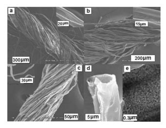
Fig. 3 SEM images of an individual fiber bundle of (a) the original cotton, (b) the coated cotton, and (c) the titania replica. Insets are enlarged images. (d) Closer SEM image and (e) TEM image of a titania microtube.
