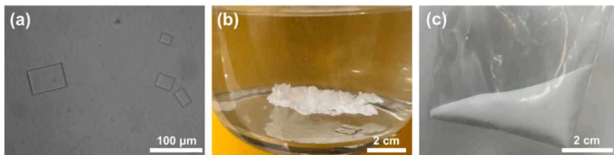
Fig. 7. (a) Crystal morphology observed under an optical microscope after 1 h of MDC; (b) white crystals formed in the crystallization tank during MDC. (c) The crystal salt after drying.
