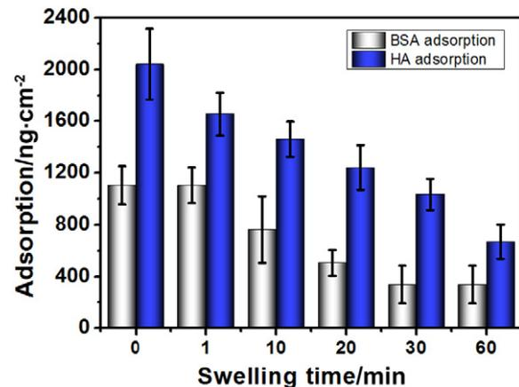
Fig. 7. BSA/HA adsorption of the SFEG membranes fabricated by swelling at 50 °C for different durations.
