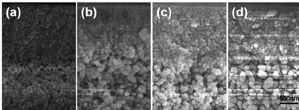
Figure 5. The cross-sectional SEM images of (a) the bare and the deposited membranes with (b) 20, (c) 40, and (d) 60 ALD cycles.
