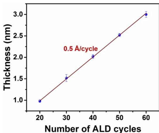
**Figure 3.** The thickness of TiO<sub>2</sub> layers deposited on silicon wafers with different cycle numbers.
