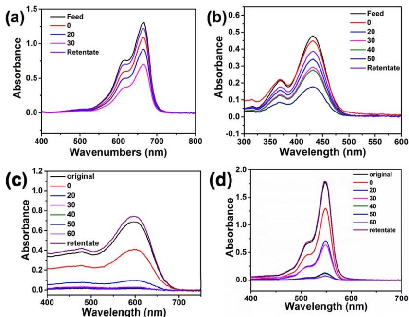
**Figure 8.** The UV-vis spectra of the feed, permeate, and retentate of (a) MB, (b) CYX, (c) RB5, and (d) RB aqueous solutions filtrated through the bare and deposited membranes with varied ALD cycles.
