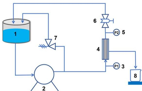
Figure 1. Schematic diagram of the filtration apparatus: (1) feed tank; (2) plunger pump; (3, 5) pressure gauge; (4) membrane module; (6) counterbalance valve; (7) safety valve and (8) beaker.
