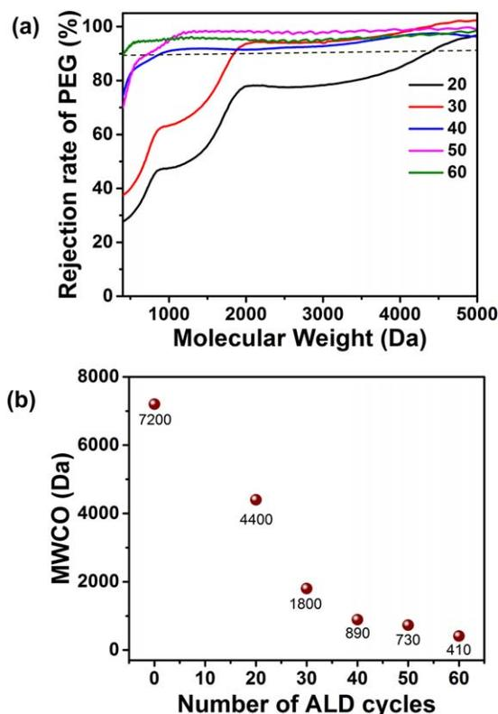
Figure 7. (a) PEG retention of the membranes with varied  $\text{TiO}_2$  deposition cycles (the dashed line indicates the rejection of 90% at which the MWCO is determined), and (b) the corresponding MWCO versus cycles.
