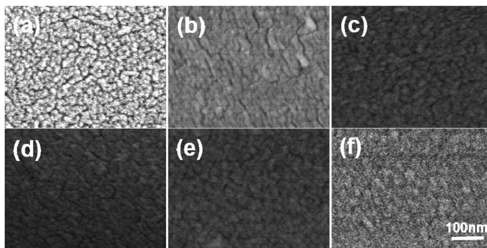
**Figure 4.** SEM images of the surface of (a) bare ceramic membrane, the TiO<sub>2</sub>-deposited membrane with cycle numbers of (b) 20, (c) 30, (d) 40, (e) 50, and (f) 60.
