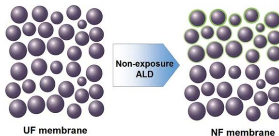
Figure 2. Schematic diagram of fabricating ceramic NF membranes from UF membranes using ALD in the nonexposure mode.
