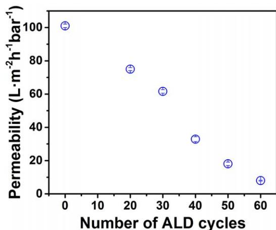
Figure 6. Water permeability of the bare membrane and the membranes with varied  $\text{TiO}_2$  deposition cycles.
