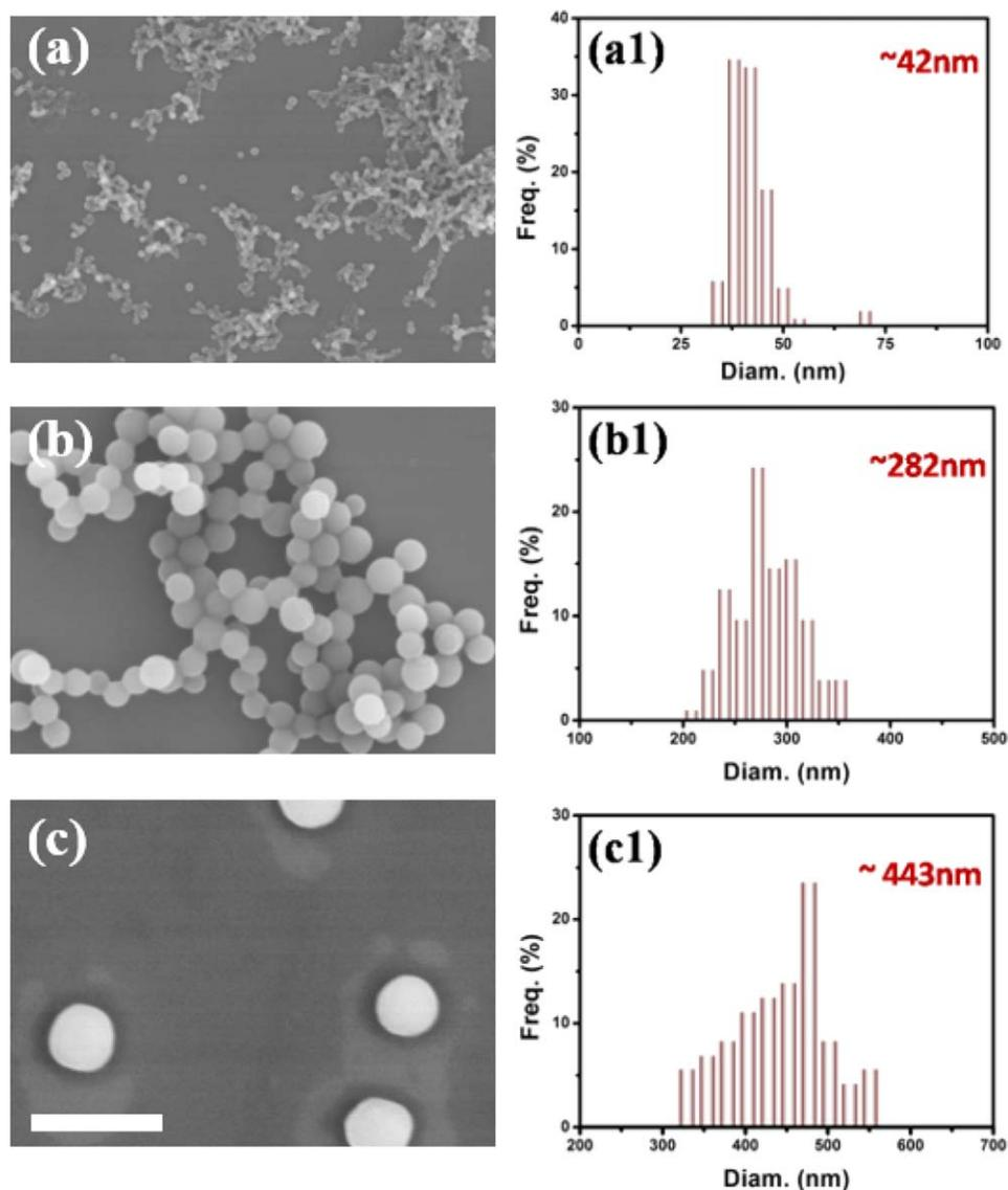
**FIGURE 6** SEM images of the FG-4 micelles prepared in AA at different temperatures: (a) 110 °C; (b) 150 °C; (c) 180 °C. (a1, b1, c1) are the corresponding size distribution histogram in 110 °C, 150 °C, and 180 °C. (a), (b), and (c) have the same magnification and the scale bar in (c) is 1000 nm. [Color figure can be viewed at [wileyonlinelibrary.com](http://wileyonlinelibrary.com)]
