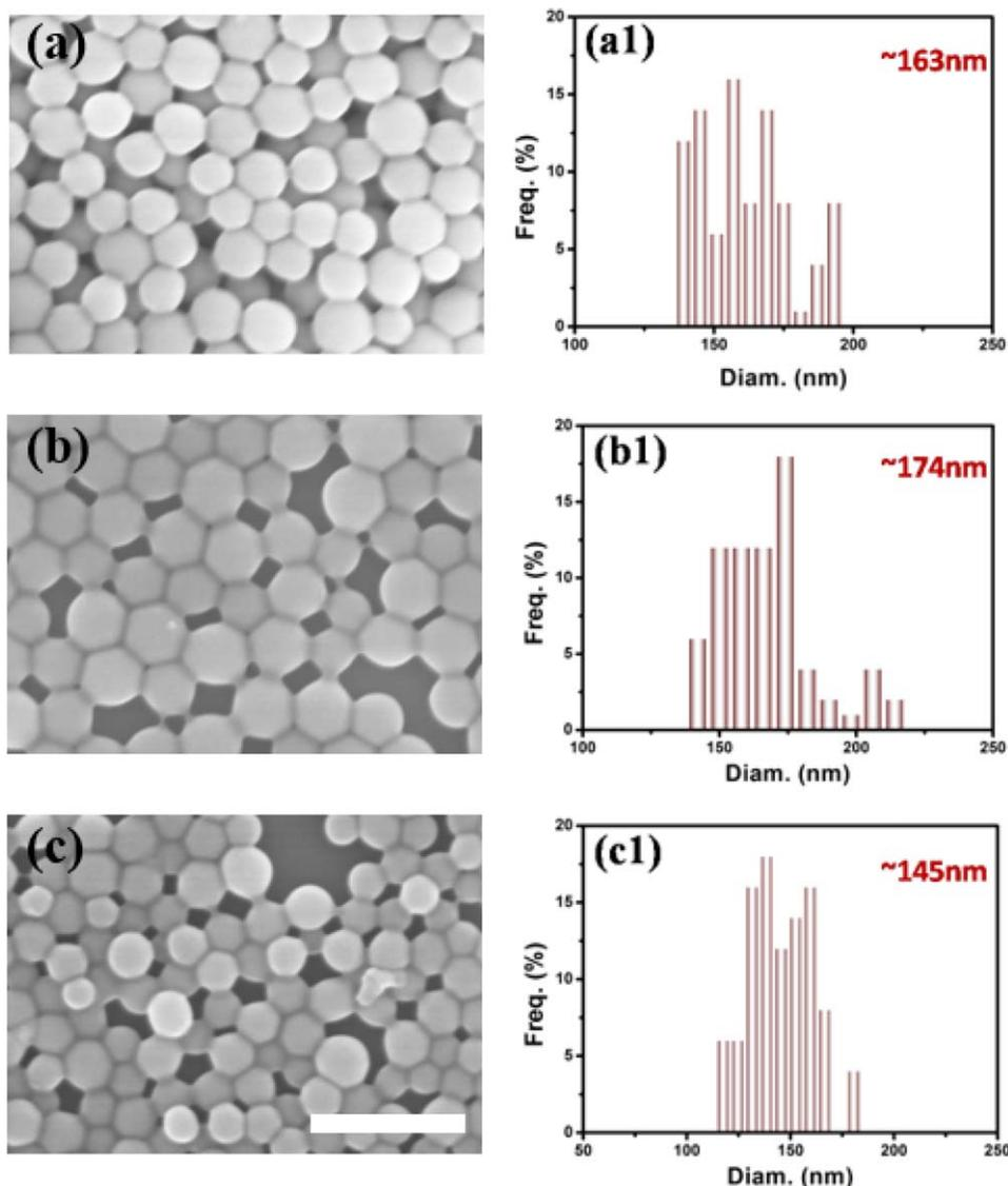
**FIGURE 5** SEM images of the PSF-*b*-PEG micelles with different PEG block ratios: (a) FG-4 (47%); (b) FG-3 (31%); (c) FG-2 (21%). (a1, b1, c1) are the corresponding size distribution histogram with different PEG block ratios. (a), (b), and (c) have the same magnification and the scale bar in (c) is 500 nm. [Color figure can be viewed at [wileyonlinelibrary.com](http://wileyonlinelibrary.com)]
