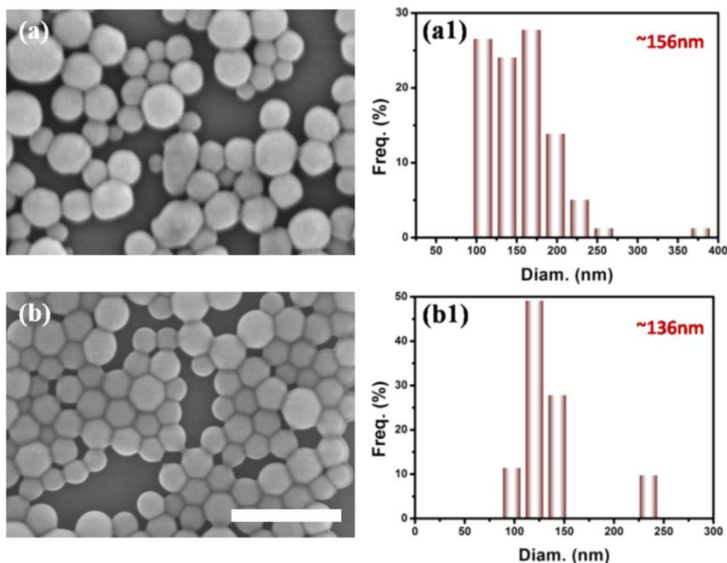
**FIGURE 4** SEM images of the FG-1 micelles and the corresponding size distribution histograms in different solvents: (a), (a1) acetone; (b), (b1) acetic acid. (a) and (b) have the same magnification and the scale bar in (b) is 500 nm. [Color figure can be viewed at [wileyonlinelibrary.com](http://wileyonlinelibrary.com)]
