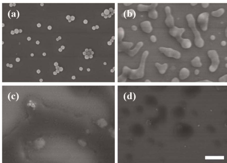
**FIGURE 8** SEM images of the FG-2 micelles after treatment at (a) 150 °C, (b) 180 °C, and (c) 200 °C for 30 min, respectively. (d) is the FG-4 micelles after treatment at 150 °C for 30 min. (a), (b), (c), and (d) have the same magnification and the scale bar in (d) is 1000 nm.
