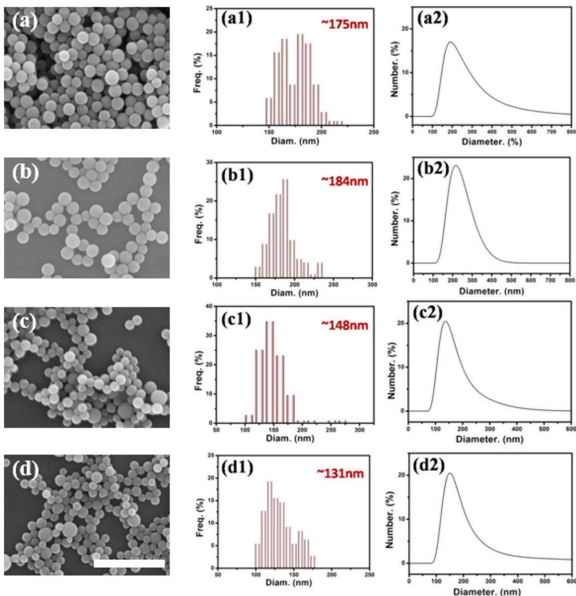
**FIGURE 7** SEM images of the PSF-*b*-PEG micelles with different PEG block ratio dispersed in deionized water: (a) FG-4; (b) FG-3; (c) FG-2; (d) FG-1. (a1, b1, c1, d1) are the corresponding size distribution histogram. (a2, b2, c2, d2) are the DLS curves of the micelles. (a), (b), (c), and (d) have the same magnification and the scale bar in (d) is 1000 nm. [Color figure can be viewed at [wileyonlinelibrary.com](http://wileyonlinelibrary.com)]
