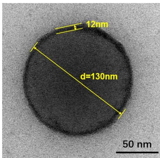
**FIGURE 3** TEM image of the FG-4 micelle after stained with  $\text{OsO}_4$ . [Color figure can be viewed at [wileyonlinelibrary.com](http://wileyonlinelibrary.com)]
