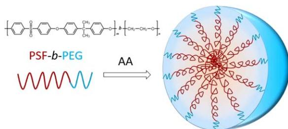
**FIGURE 1** The schematic diagram of the formation of PSF-*b*-PEG spherical micelle with core-shell structure through direct dissolving method. [Color figure can be viewed at wileyonlinelibrary.com]
