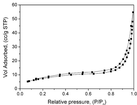
**Figure 6.** Nitrogen sorption isotherm for the microflowers obtained with an etch time of 36 h.
