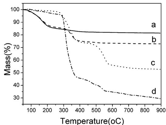
**Figure 5.** TG curves of original zeolite (a), PS/zeolite composite (b), and composite treated with HF for 36 h (c) and 120 h (d).
