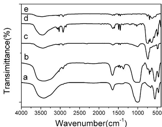
**Figure 4.** FTIR spectra of original zeolite (a), PS/zeolite composite (b), and composites treated with HF for 5 h (c), 36 h (d), and 120 h (e).
