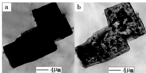
**Figure 8.** TEM images of  $\text{Na}_2\text{SiF}_6$  crystals before (a) and after (b) exposure to electron beam for about 20 s.
