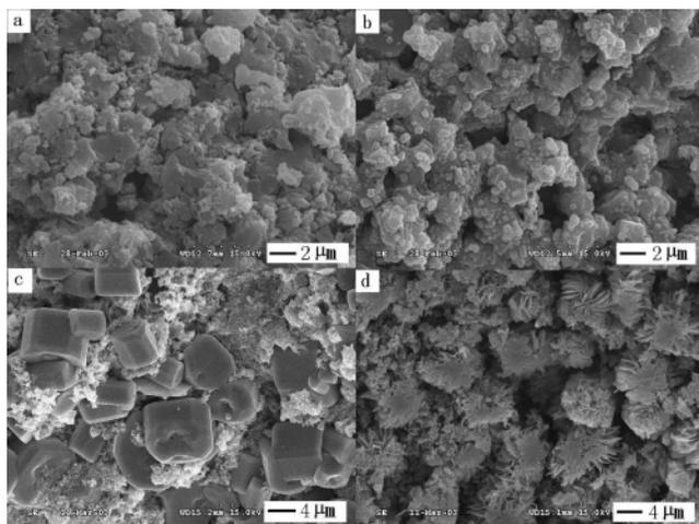
**Figure 7.** SEM images at different stages of the preparation of microflowers. (a) The original zeolite, (b) the PS/zeolite composite, and composites treated with HF solution for 5 h (c) and 24 h (d).
