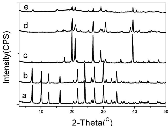
**Figure 3.** XRD patterns of original zeolite (a), PS/zeolite composite (b), and composites etched with HF for 5 h (c), 36 h (d), and 120 h (e).
