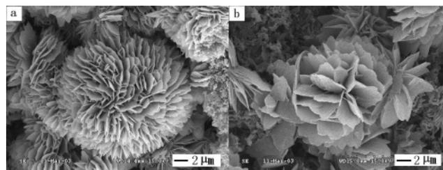
**Figure 9.** Flowerlike structures prepared from composites of zeolite and PMMA (a) and PDVB (b).
