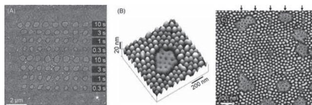
**Figure 6.** Atomic force microscopy images of PS-*b*-P2VP micellar films with micelles on some areas opened by glycerol droplets locally dispersed by an AFM cantilever. A) Array of spots made of opened micelles after exposure to glycerol droplets. The contact times of the AFM cantilever for each line are noted on the left-hand side. B) Detail of one of the smaller spots. C) Some well-recognizable individual opened micelles. Reproduced with permission.<sup>[70]</sup> Copyright 2006, Elsevier.
