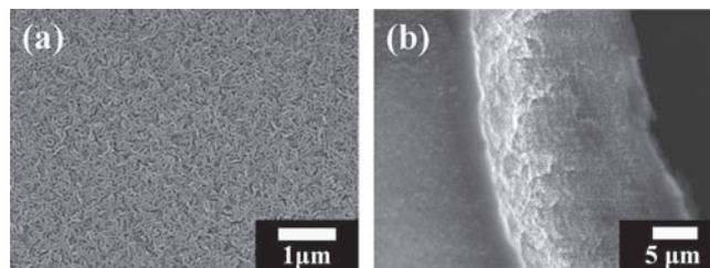
**Figure 8.** Scanning electron microscopy images of a PS-*b*-P2VP bulk film with a thickness of tens of micrometers immersed in ethanol at 60 °C for 15 h. It has interconnected nanopores throughout the entire film: a) top surface and b) cross section.
