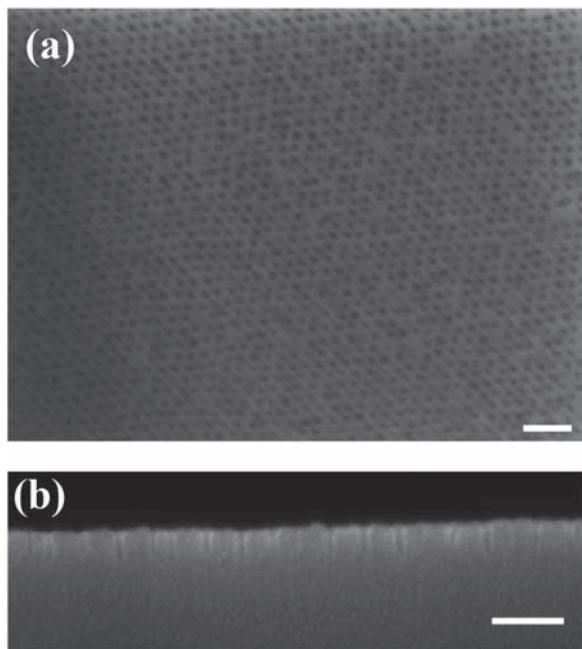
**Figure 4.** Scanning electron microscopy images of highly ordered arrays of nanopores fabricated on the silicon substrate via reactive ion etching through an etching mask of a gold-coated, reconstructed PS-*b*-P4VP film: a) top view and b) cross-sectional view. A thin layer of gold was evaporated on the surface of the BCP film to enhance the etching contrast with silicon. The scale bar represents 100 nm. Adapted with permission.<sup>[68]</sup> Copyright 2008, American Chemical Society.
