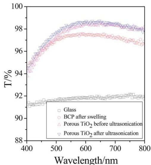
**Fig. 6** The transmittance spectra of the porous BCP membrane prepared by spincoating the 0.6% BCP solution on the glass substrate followed by swelling at 65 °C for 15 h and the TiO<sub>2</sub> membrane prepared by ALD deposition of TiO<sub>2</sub> on the above-mentioned BCP membrane with 60 cycles before and after the ultrasonication treatment.
