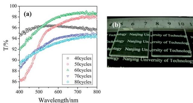
**Fig. 5** (a) Transmittance spectra of porous TiO<sub>2</sub> membranes prepared from a BCP template with different numbers of ALD cycles. (b) The photograph of a bare glass substrate (left) and a glass substrate with a TiO<sub>2</sub> membrane coating layer prepared at 60 ALD cycles (right).
