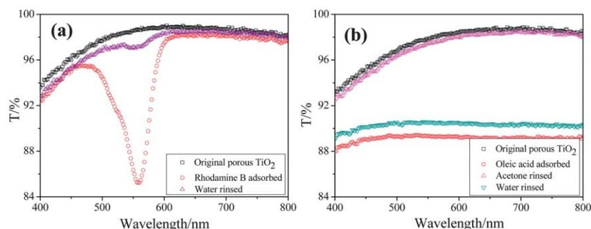
**Fig. 7** Transmittance spectra of the porous TiO<sub>2</sub> membrane prepared at an ALD cycle number of 60 contaminated by the adsorption of Rhodamine B and cleaned by rinsing with water (a), and transmittance spectra of this porous TiO<sub>2</sub> membrane contaminated by the adsorption of oleic acid and cleaned by rinsing with acetone (b).
