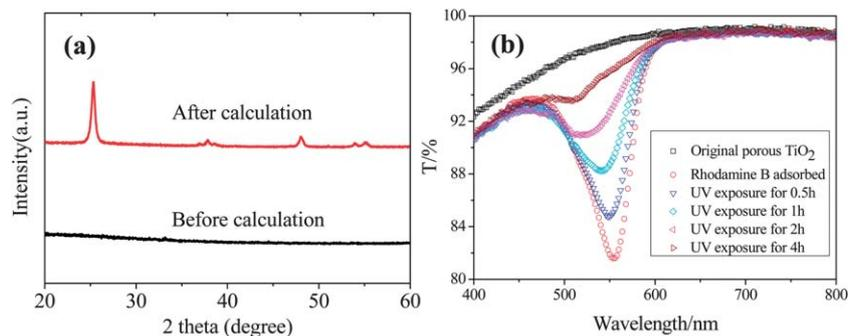
**Fig. 8** (a) XRD patterns of the porous BCP membrane subjected to 80 TiO<sub>2</sub> ALD cycles before and after calcination in air at 450 °C. (b) Transmittance spectra of the porous TiO<sub>2</sub> membrane prepared at an ALD cycle number of 60 contaminated by the adsorption of Rhodamine B and cleaned by UV exposure for different times.
