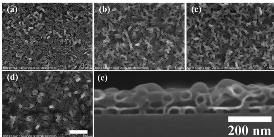
**Fig. 4** SEM images of the surface (a–d) and cross-section (e) of porous  $\text{TiO}_2$  networks prepared by ALD on BCP templates with different ALD cycle numbers: (a) 40 cycles, (b) 50 cycles, (c and e) 60 cycles, (d) 70 cycles. The BCP templates were prepared by spincoating the 0.6% BCP solution on glass substrates followed by swelling at 65 °C for 15 h. Panels (a–d) have the same magnification and an additional enlarged scale bar corresponding to 500 nm is shown in (d).
