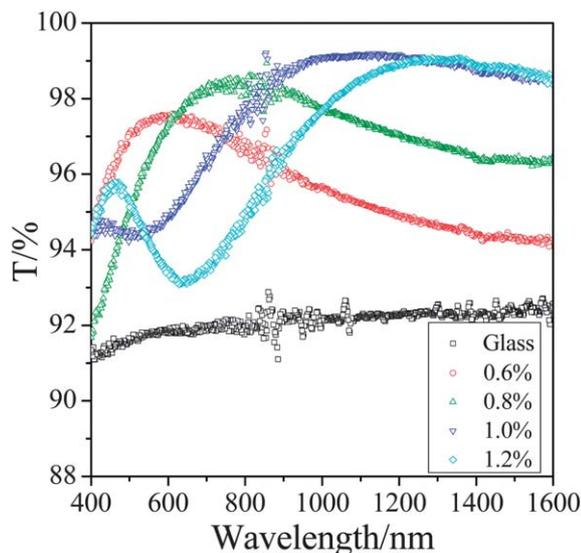
**Fig. 2** Transmittance spectra of the porous BCP membranes prepared with different BCP concentrations.
