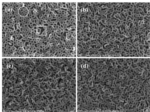
**Fig. 1** SEM images of the surface morphology of porous membranes obtained from BCP solutions with different concentrations: (a) 0.6%; (b) 0.8%; (c) 1.0%; (d) 1.2%. The porous membranes were prepared by swelling the spincoated BCP films in ethanol at 65 °C for 15 h, followed by air drying at room temperature.
