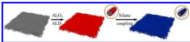
**Figure 1.** Hydrophobization process of filter papers including atomic layer deposition of  $\text{Al}_2\text{O}_3$  and silane coupling.
