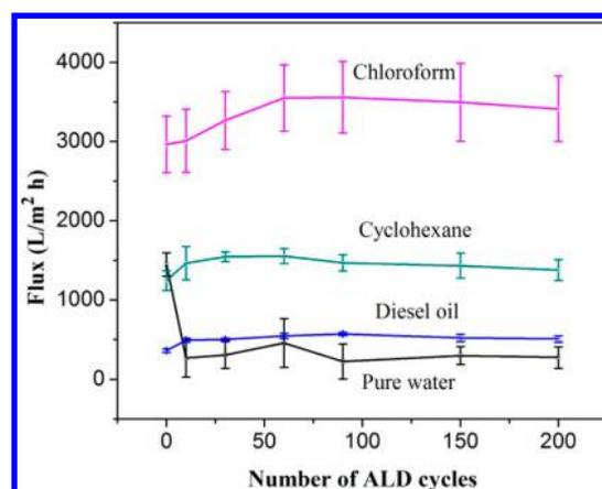
**Figure 6.** Flux of pure water, cyclohexane, diesel oil, and chloroform for filter papers as a function of different ALD cycle numbers.
