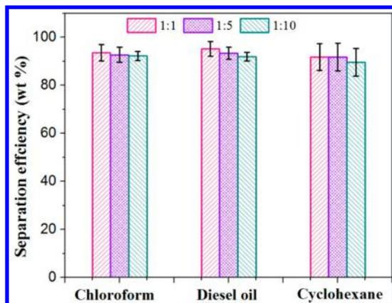
**Figure 8.** Separation efficiencies of the modified filter papers for different oil/water mixture systems (oil:water mass ratio = 1:1, 1:5, 1:10).
