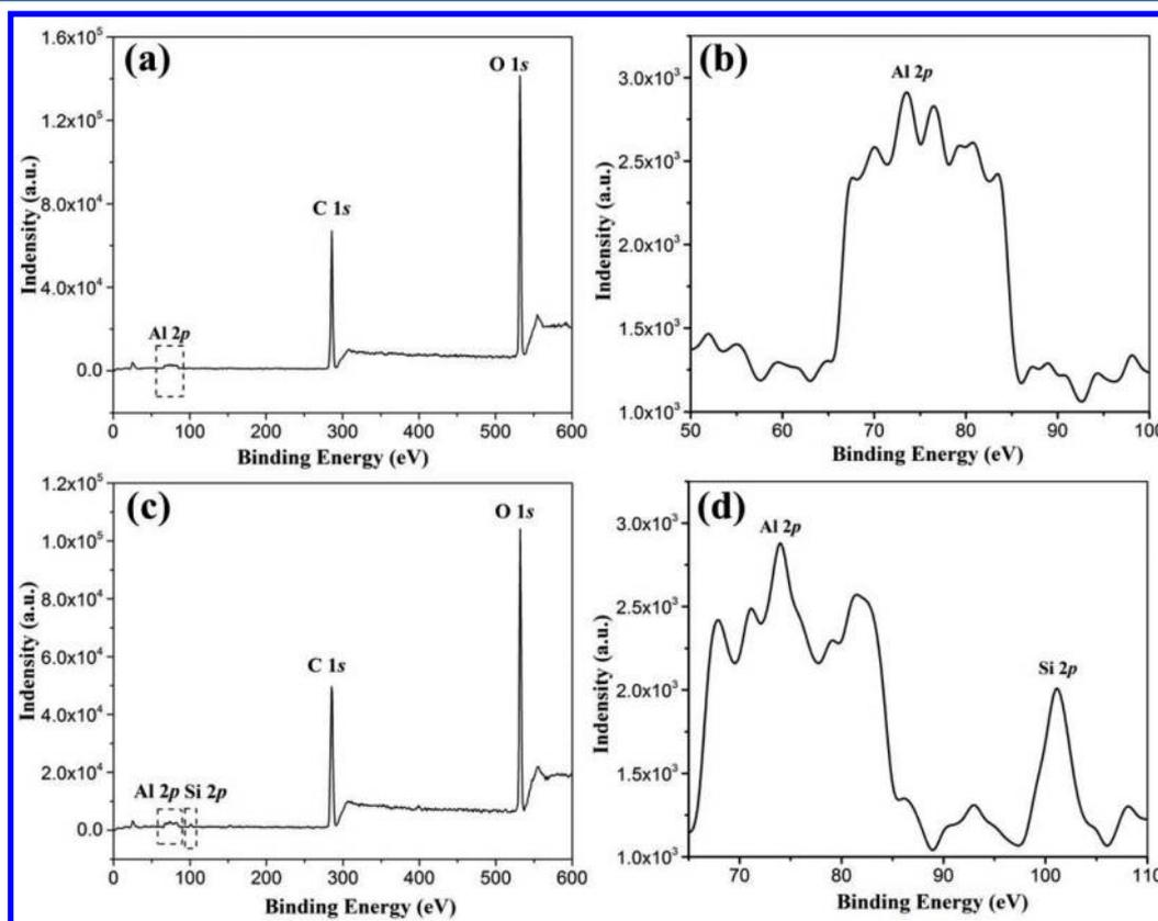
**Figure 2.** XPS spectra of the  $\text{Al}_2\text{O}_3$ -deposited filter paper (a: survey and b: Al  $2p$ ) and the silanized filter paper after  $\text{Al}_2\text{O}_3$  deposition (c: survey and d: Al  $2p$  and Si  $2p$ ).
