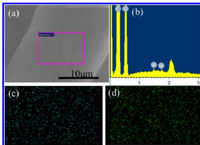
**Figure 3.** EDS analysis of the modified filter paper with 90 ALD cycles and silanization: (a) the selected area; (b) surface scanning spectrum; (c) surface distribution of Si; and (d) surface distribution of Al in the scanned area marked in (a).
