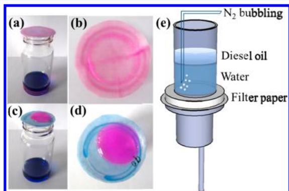
**Figure 7.** Photographs showing the separation and wetting behavior of a diesel oil (blue)/water (red) mixture using pristine filter paper (a: overall, b: top view), modified filter paper (c: overall, d: top view), and the diagram of the filtration cell (e) showing the experimental setup of the separation process for the mixture of water and diesel oil. The sample used in Figure 8c and d was the modified filter paper with 90 ALD cycles followed by KH-570 coupling.
