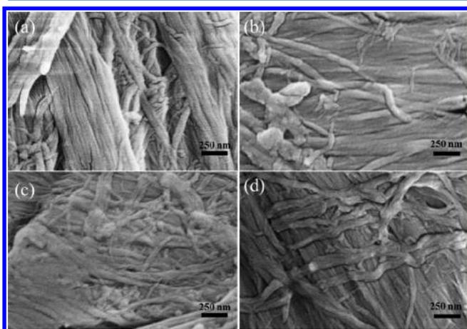
**Figure 4.** Surface SEM images of filter paper before (a) and after  $\text{Al}_2\text{O}_3$  deposition with 90 (b) and 200 (c) ALD cycles and silanization after 90 ALD cycles (d).
