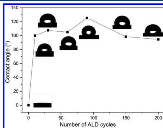
**Figure 5.** Average water contact angles measured on filter papers before and after different ALD  $\text{Al}_2\text{O}_3$  cycles. The insets show the photographs of the water droplet on the filter paper.
